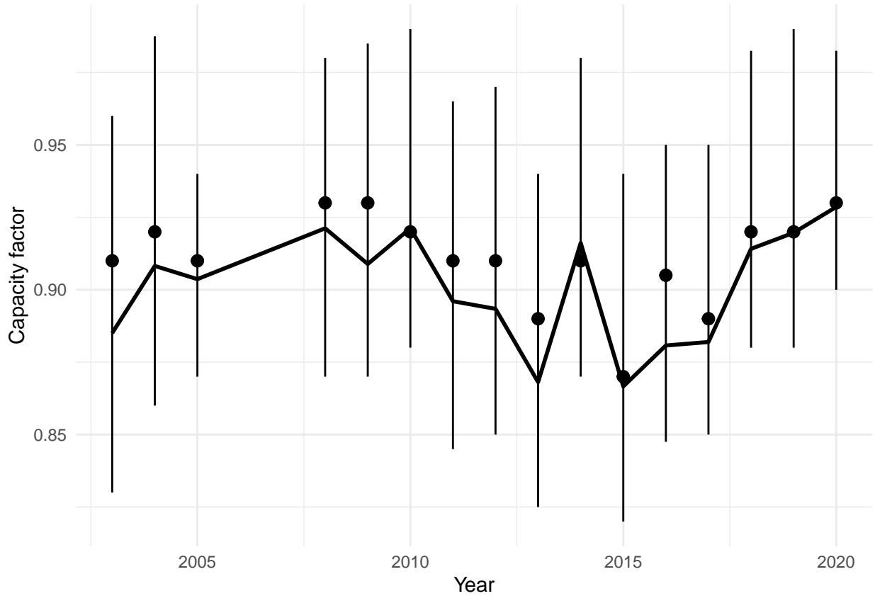
Figure A.8: Capacity factors of US nuclear power plants by year. The figure plots mean (solid line) and median (points) capacity factor, by year. The vertical lines correspond to the interquartile range, marking the 25th and 75th percentiles. Data for 2006, 2007, and years prior to 2003 were not reported by the NRC.
